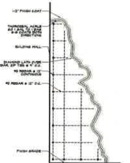
1 FAUX ROCK DETAIL SCALE: 1/2"=1'-0"
