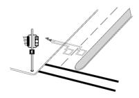
loops placed in the pavement at intersections.
