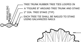
NOTE: MINIMUM (2) TIES (TOP & BOTTOM) REQUIRED. USE A THIRD TIE WHEN NECESSARY TO KEEP TREE UPRIGHT POSITION. TIES TO BE SECURED TO AVOID SLIPPAGE. WRAP STAKE TO FORM FIGURE EIGHT, SCREW W/ 1 GALV. SCREW THROUGH EACH TIE INTO POLE
