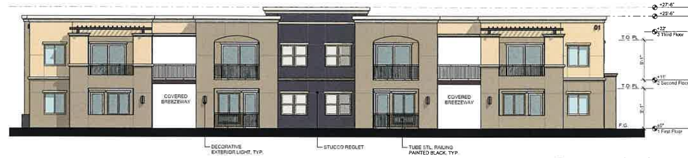
03 Bldg 1 - South Elevation SCALE: 1/8" = 1'-0"
