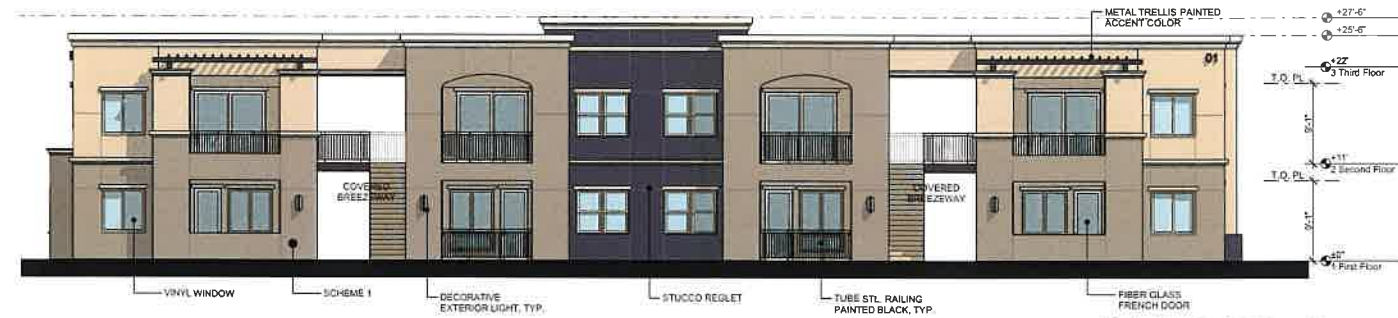
01 Bldg 1 - North Elevation SCALE: 1/8" = 1'-0"
