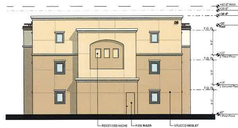
04 Bldg 8 - South Elevation SCALE: 1/8" = 1'-0"
