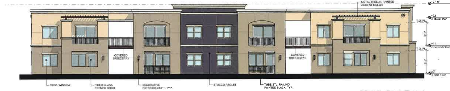
03 Bldg 9 - South Elevation SCALE: 1/8" = 1'-0"
