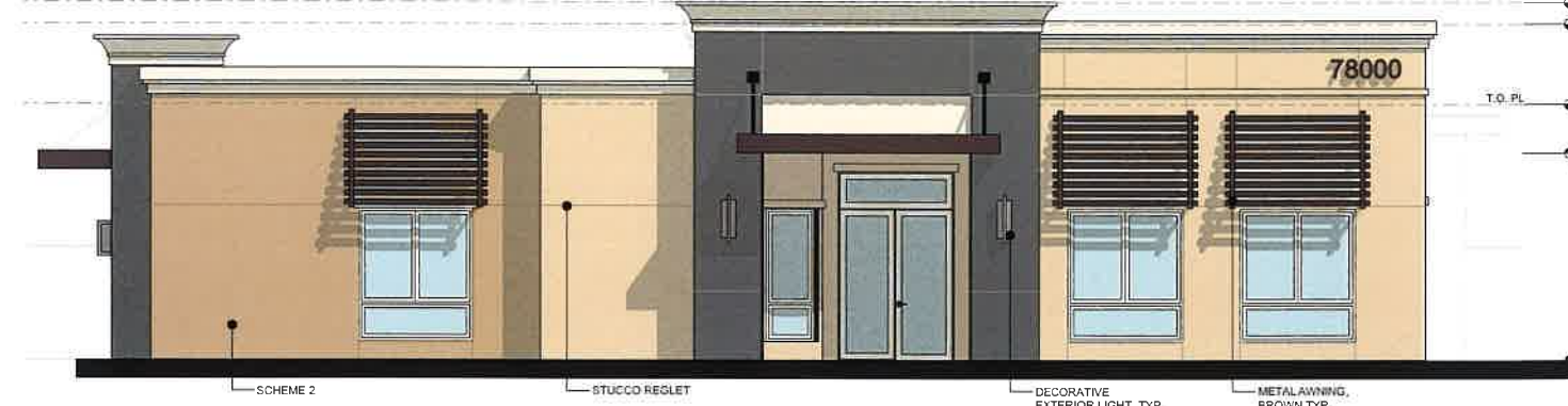
01 Clubhouse - West Elevation (Entry) SCALE: 1/4" = 1'-0"
