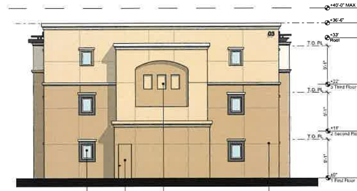
02 Bldg. 3 - South Elevation SCALE: 1/8" = 1'-0"
