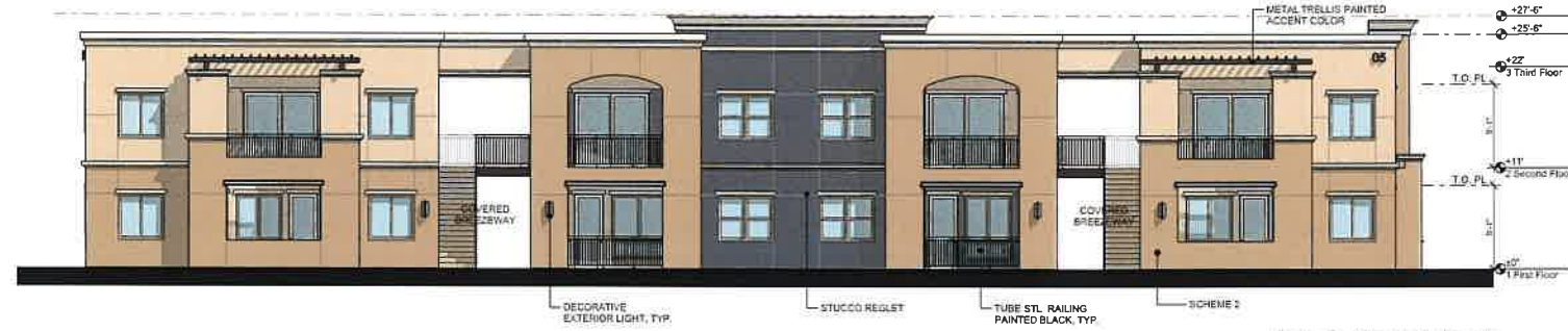
01 Bldg 5 - North Elevation SCALE: 1/8" = 1'-0"
