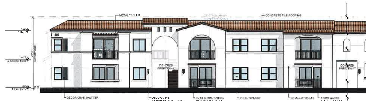
03 Bldg 4 Front Elevation B SCALE: 1/8" = 1'-0"
